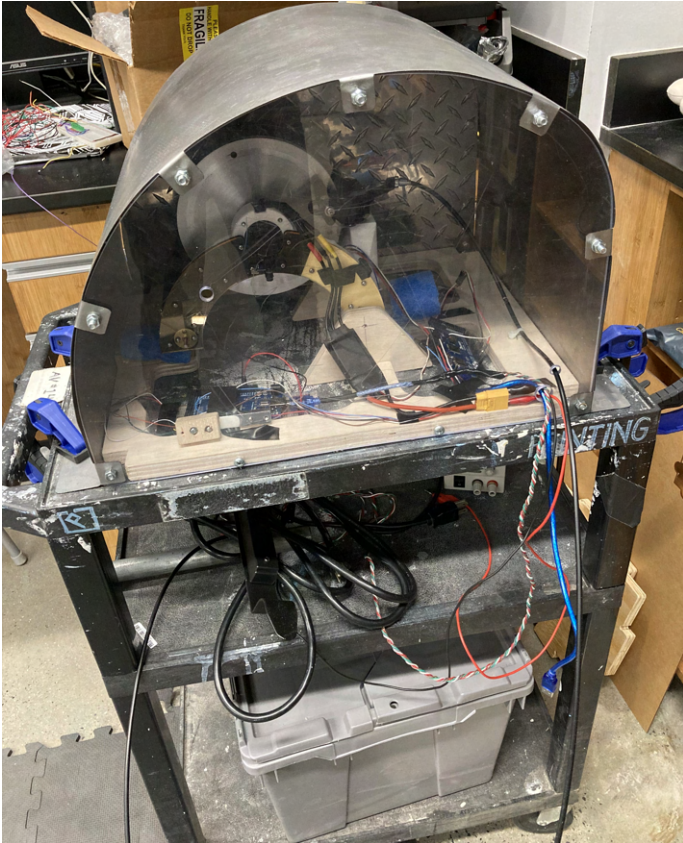
FIGURE 11. Test stand fully assembled and all instrumentation in place.
