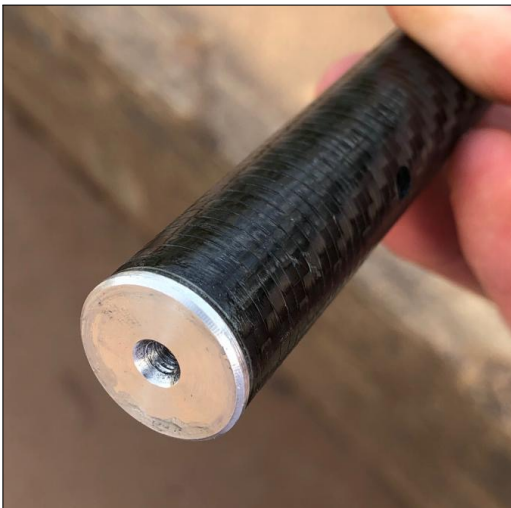
Fig. 24 Endcaps Epoxied into Spars
